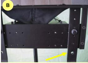
Remove both CRT support arms - these are fastened from the back with allen head screws.
