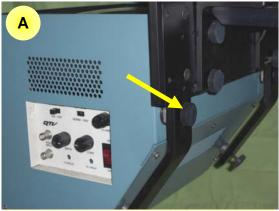
Start by removing the old CRT. There are 2 thumbnuts to unscrew - they can be used to mount the new display.
