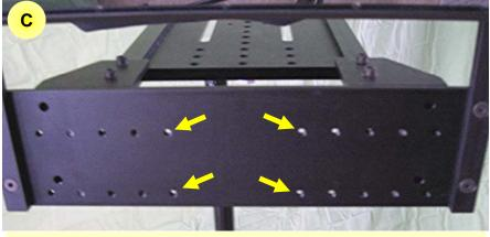
Use a 1/4" drill bit to clear the threads from the four centermost holes in the backplate - these are the mounting holes for the new LCD display.
